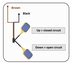
For greater differential, dual floats can be attached on the source inputs 5, 6 and 7. (COM, L1, L2)
