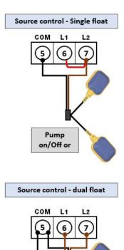
3 wire' floats allow for NO or NC wiring.
