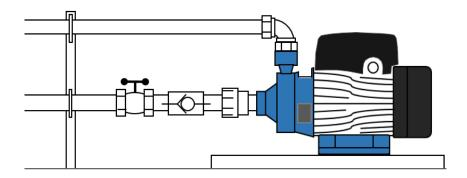
Mount the pump on a firm base in a dry, free draining area Protect the pump from weather, dust, insects and extremes of temperature
