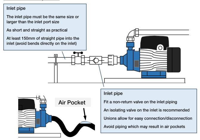
The pump and delivery line MUST be manually primed (filled) before the pump is started for the first time to ensure the mechanical seal is well lubricated. Dry operation causes irreparable damage to the mechanical seal.
